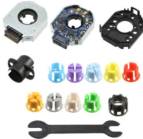
**MA3 magnetic encoder** comes in 10 bit and 12 bit version (10bit has 1kHz refresh rate, 12bit has 244Hz refresh rate). <http://www.usdigital.com/products/encoders/absolute/rotary/shaft/MA3>
